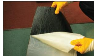
3. Peel off protective film under the coating
